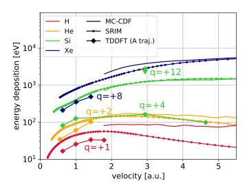
FIG. 4. Energy deposition in graphene for different projectile ion species and velocities. Results from TDDFT (diamonds), MC-CDF (solid curves), and SRIM (circles) are compared. The text annotations correspond to the initial charge states of the ions in TDDFT; the MC-CDF calculations use an equilibrium effective charge given by the Barkas formula [30].
