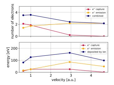
FIG. 7. (a) Number of electrons emitted and captured in TDDFT for  $Si^{+4}$  ions of varying velocities. (b) Total energy deposited and dissipated via electron emission and electron capture for  $Si^{+4}$  ions of varying velocities in TDDFT simulations.
