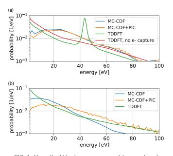
FIG. 5. Normalized kinetic-energy spectra of the secondary electrons emitted from graphene after impact by (a)  $H^+$  80 keV and (b) Si<sup>+4</sup> 15 MeV. TDDFT with (green) and without (red) captured electrons is compared to MC-CDF before (blue) and after (orange) including PIC simulations. MC-CDF results were computed with the Barkas effective charge [30].
