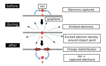
FIG. 1. Schematics of the electron dynamics before (top), during (middle), and after (bottom) the impact of a SHI in graphene. The approximate timescale of the dynamics shown here is on the order of femtoseconds.
