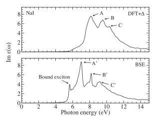
FIG. 2. Imaginary part of the dielectric function  $\epsilon(\omega)$  computed using the DFT +  $\Delta$  approximation (top) as well as the BSE approach (bottom) for NaI.
