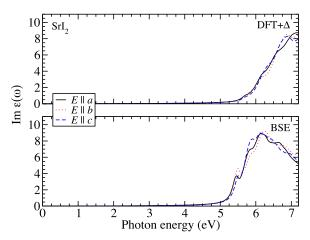
FIG. 5. Imaginary part of the dielectric function  $\epsilon(\omega)$  computed using the DFT +  $\Delta$  approximation (top) as well as the BSE approach (bottom) for SrI<sub>2</sub>. The optical anisotropy is shown for both.
