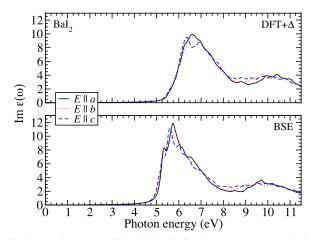
FIG. 4. Imaginary part of the dielectric function  $\epsilon(\omega)$  computed using the DFT +  $\Delta$  approximation (top) as well as the BSE approach (bottom) for BaI<sub>2</sub>. The optical anisotropy is shown for both.
