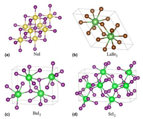
FIG. 1. Unit cells of the materials studied in this work: (a) NaI, (b) LaBr<sub>3</sub>, (c) BaI<sub>2</sub>, and (d) SrI<sub>2</sub>.
