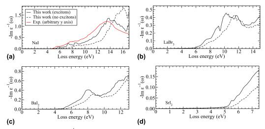
FIG. 7. Electron-energy loss function  $-\text{Im }\epsilon^{-1}(\omega)$  computed from the dielectric function including (solid lines) and excluding (dashed lines) excitonic effects, according to Eq. (1) for NaI (a), LaBr<sub>3</sub> (b), BaI<sub>2</sub> (c), and SrI<sub>2</sub> (d). For NaI, a measured curve <sup>68</sup> is included for comparison.
