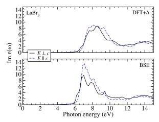
FIG. 3. Imaginary part of the dielectric function  $\epsilon(\omega)$  computed using the DFT +  $\Delta$  approximation (top) as well as the BSE approach (bottom) for LaBr<sub>3</sub>. The optical anisotropy is shown for both.
