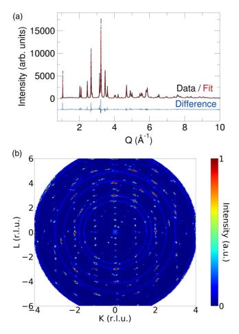
FIG. 2. The Rietveld-refined fit to the synchrotron powder x-ray diffraction data of Fe<sub>2</sub>As is shown in (a). The elastic neutron scattering slice along K and L for H integrated from -0.2 to 0.2 is shown in (b) for  $E_i = 30$  meV.
